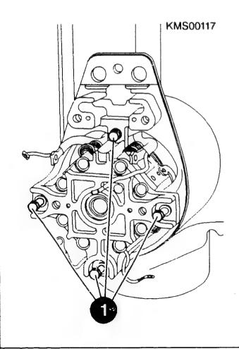
STARTING-MOTOR DISASSEMBLY Disassembling intermediate bearing Clamp armature in clamping support. Slip centering sleeve (1) onto drive spindle. Use commercially available jaw-type puller to remove deep-groove ball bearing from bearing end plate. Clamping support: 0 986 619 362 Jaw-type puller: comm. avail. Centering sleeve for jaw-type puller: (improvisation)
